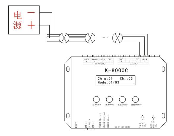
1. Like the above diagram, wired the line and start the controller, press "CHIP" and "MODE" at the
