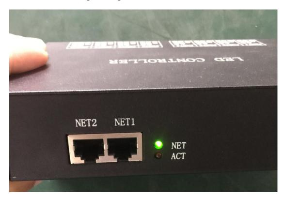
Connect NET1 to computer network interface with RJ45
