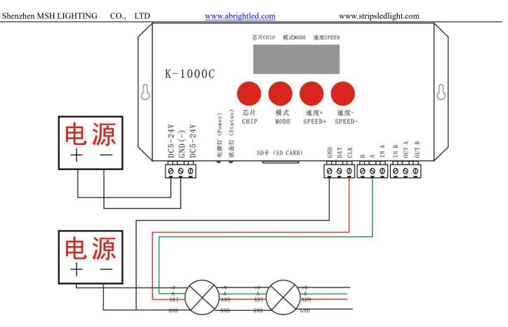
1. Like the above diagram, wired the line and start the controller, press "CHIP" and "MODE" at the same time switch to coding mode, adjust to Chip: 61 that is UCS512A or B coding mode, as below:
