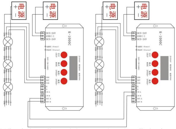
NOTE:1. When multiple controllers cascade, beginning from the second controller digital screen display 222, and status lights: on, off, on, off, strobe, all cascade controllers' playback speed controlled by the first set.
