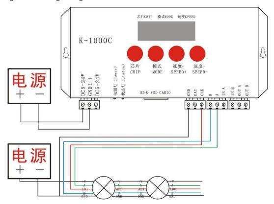
Single signal wiring diagram:
